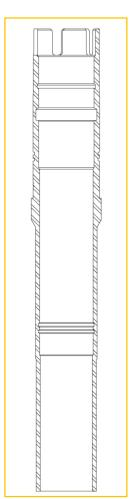
Specifications and Dimensions for Drop Off Mandrel & Tie Back Receptacle
